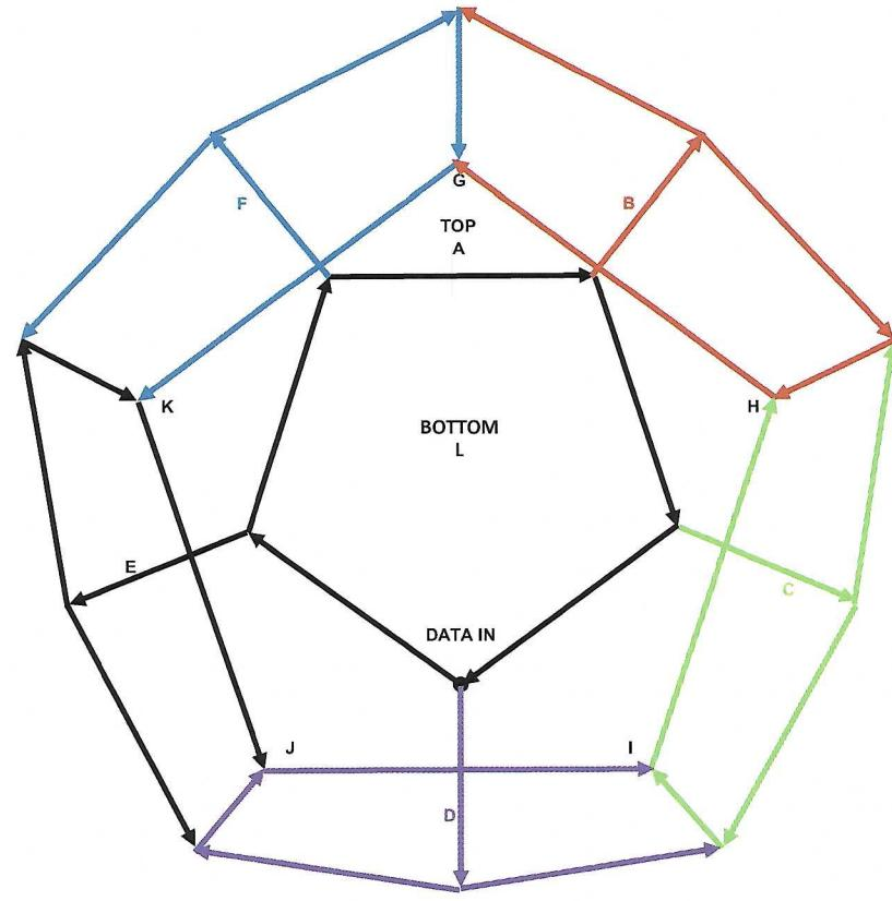
EDGE ORDER: AB, AC, AD, AE, AF, BC, CD, DE, EF, FB, BG, BH, CH, CI, DI, DJ, EJ, EK, FK, FG, GH, HI, IJ, JK, KG, GL, HL, IL, JL, KL
