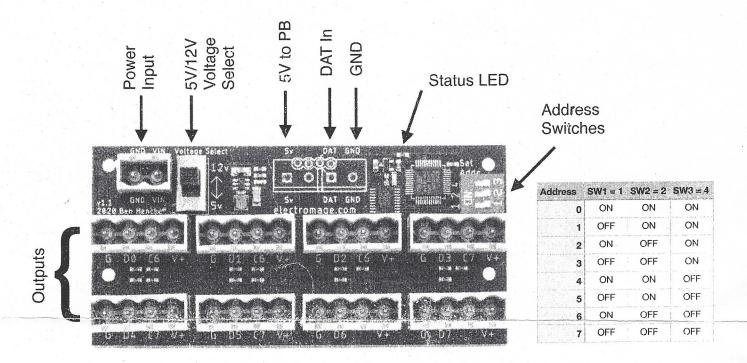
There are two input connection options. The driver board has both a 0.1" and a 0.2" header with the same electrical connections. This allows standard 0.1" pin headers or 5mm screw terminals. The board may also be soldered directly to Pixelblaze.
